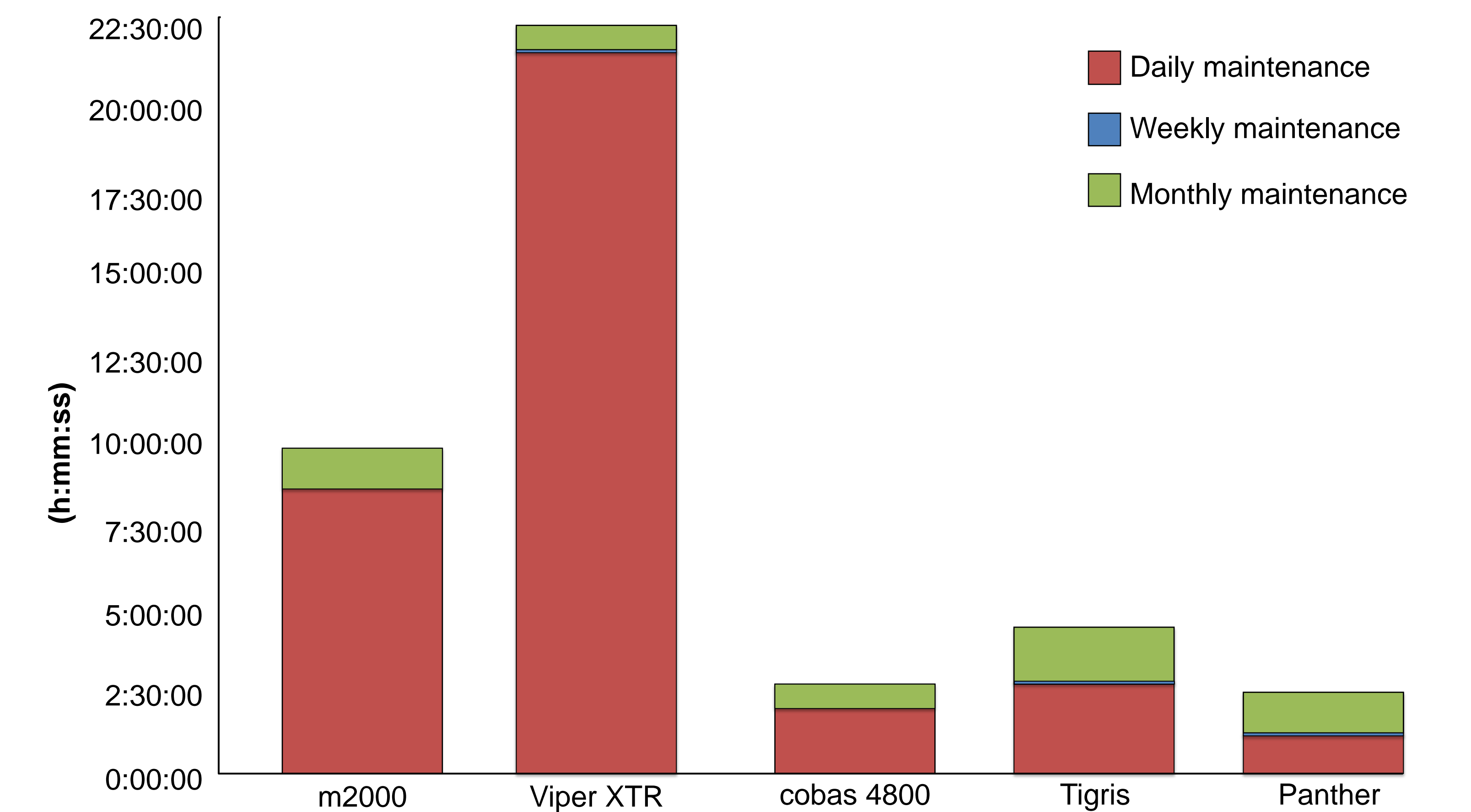
Figure 4: Cumulative hands-on time for maintenance based on 96 tests per day, 20 days per month. (Viper XTR required the most hands-on time for daily maintenance and Panther the least.)
